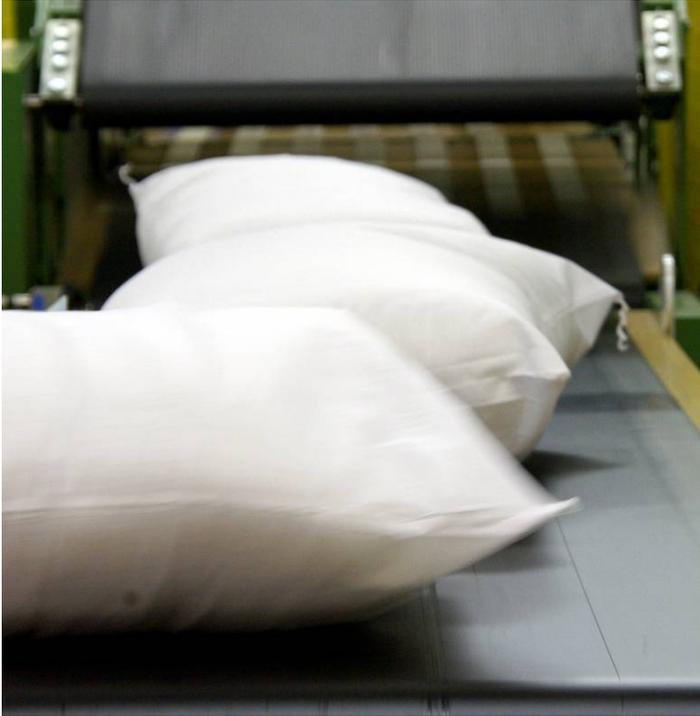
along two sides. This is then cut to the correct length and sewn along the remaining two sides. It is then weighed, rolled and packed.
